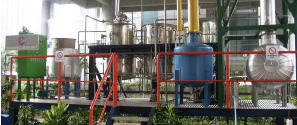
Gambar 13 Prototype Pilot Plant Kapasitas 250 liter/ batch (1,5 ton/hari) milik BPPT (Sumber: Dokumentasi Koleksi BTBRD, BPPT)
