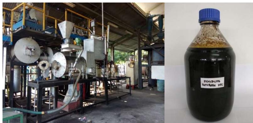
Gambar 17. Peralatan low temperature carbonization assay dan hasil syncrude
